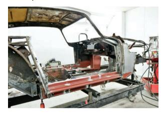
Objective – to remove all components, filth, materials, coverings and paint which is required prior to separation of the outer body shell from the chassis assembly. First stage of the strip is to remove all interior trim and glass, labelling and carefully storing. Next follows bumpers, all bright trim, light fittings etc. Next the transmission tunnel is removed followed by the removal of radiators, engine and transmission in unit, initially to be stored and later assessed.
